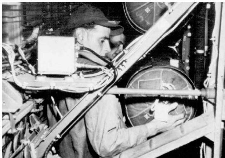
Containers, with parachute packs attached, are stored in the bomb racks within the B-24 aircraft
